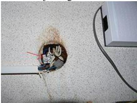
Result improperly joined aluminum and copper wires in old USSR apartments, done by qualified electrician
